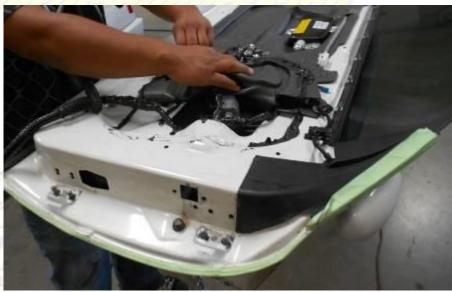
Install the provided door bracket as show in the image below. Then use a "Punch or marker" to mark the location of the holes on the door. You will need to drill new holes to allow the bolts to go through the door.
