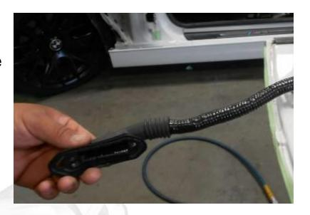
Use the provided wire harness plate with the factory 8mm bolt as shown to secure the wire harness to the body.
