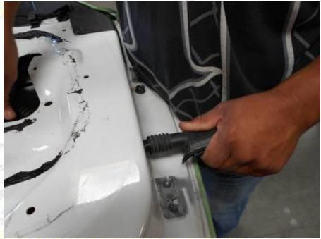
Use zip ties to secure the wires back to the door as shown.
