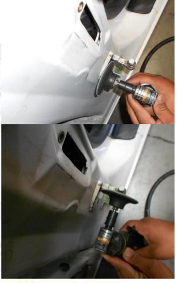
remove the door panel and peal back the door cover as shown this will allow you to remove the door catch and modify the door wiring to gain extra wire slack.
