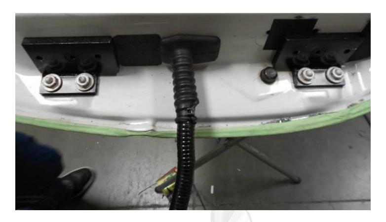
Now install the new VDI hinge system to the door as shown.
