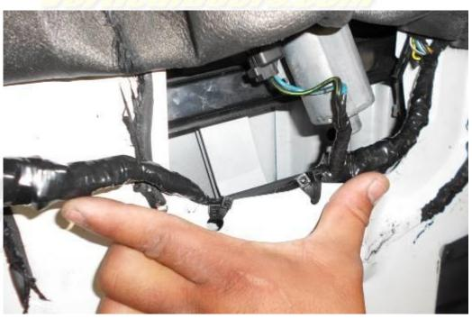
Cut the factory wire boot in half and use the provided wire loom to protect the exposed wires. Use a zip tie to secure the wire boot to the wire loom as shown.
