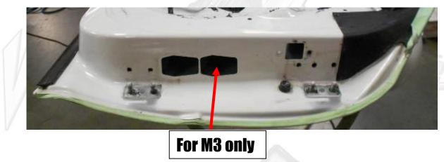
After making the new holes in the door reinstall the brackets as shown in the image below.
